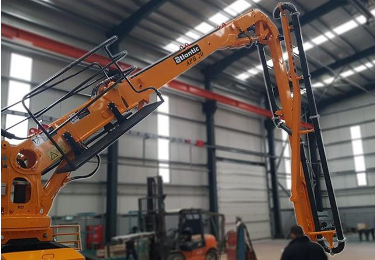
Featuring a compact structure, the Atlantic Concrete Placing Boom can be lifted and transferred to any suitable place for concrete placement, such as floors, platforms, simply-structured racks or even trailers.
